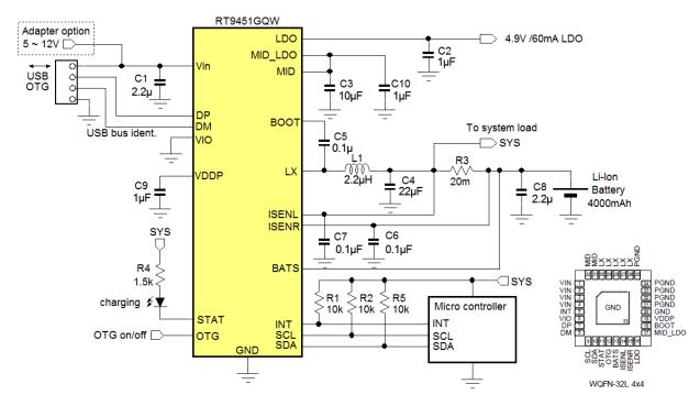
Figure 10. Typical RT9451 application for charging high capacity battery cells.
