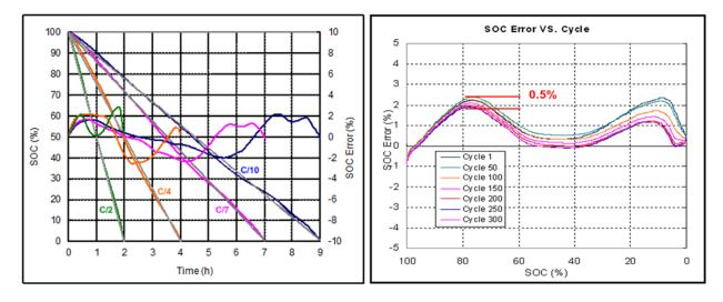
Figure 12. SOC measurement and SOC error at different discharge conditions and over charge/discharge cycles.
