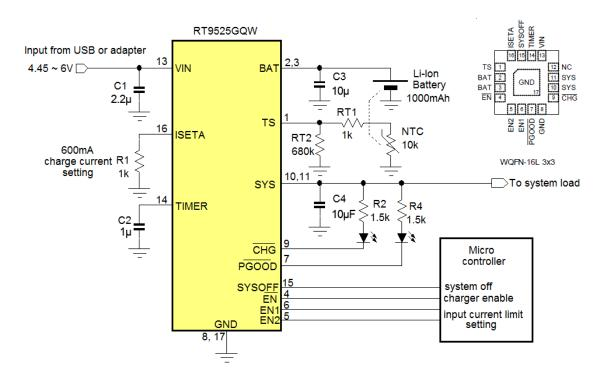
Figure 9. Typical RT9525 charger for small battery powered application with auto power path.
