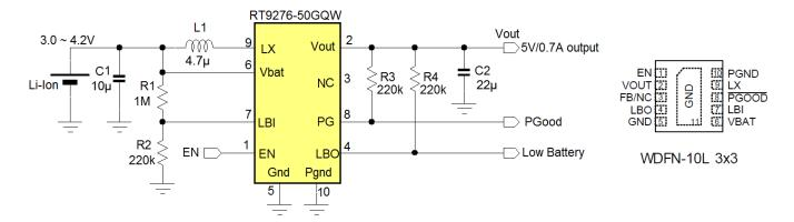
Figure 5. RT9276-50 application provides stable 5V from battery input.
