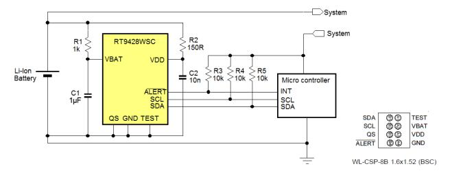
Figure 11. RT9428 battery gauge application
