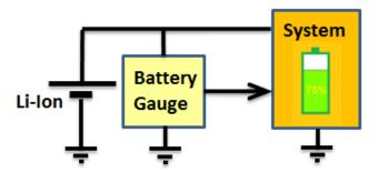
In many battery applications it is important to know how much charge is left in the battery. Checking the state of charge (SOC) of Li-lon cells is often done by coulomb counting method, which measures the battery current over time and determines the SOC from the net increase / decrease in charge. These methods are accurate in theory, but suffer from accumulation errors over time, and the circuit is complicated due to the current sense circuit.
