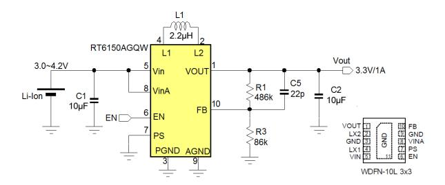
Figure 6. RT6150A automatically switches from buck to boost mode when battery drops below VOOUT.
